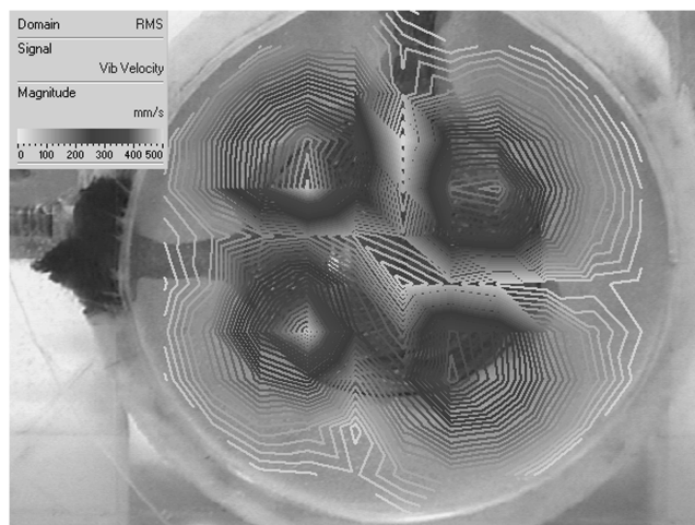
Fig. A6 Vibrometer scan at the sixth detected resonant frequency at 284 Hz excitation and 285 Hz vibration with a maximum rms vibrational velocity of 0.499 m/s at four points. Induced nozzle velocity is \pm 4 m/s.
