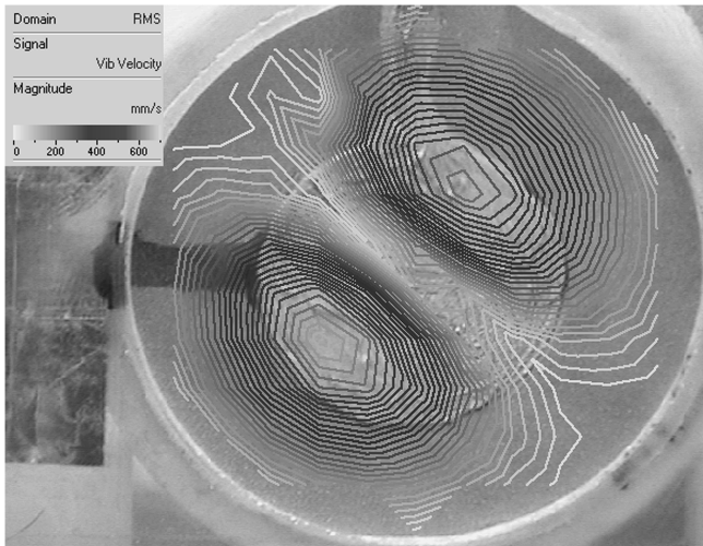
Fig. A20 Vibrometer scan at the second detected resonant frequency at 365 Hz excitation and 183.6 Hz vibration with a maximum rms vibrational velocity of 0.677 m/s at two points.
