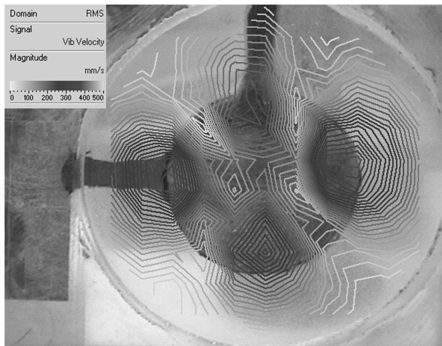
Fig. A17 Vibrometer scan at the fifth detected resonant frequency at 569 Hz excitation and 285.2 Hz vibration with a maximum rms vibrational velocity of 0.403 m/s at four points.
