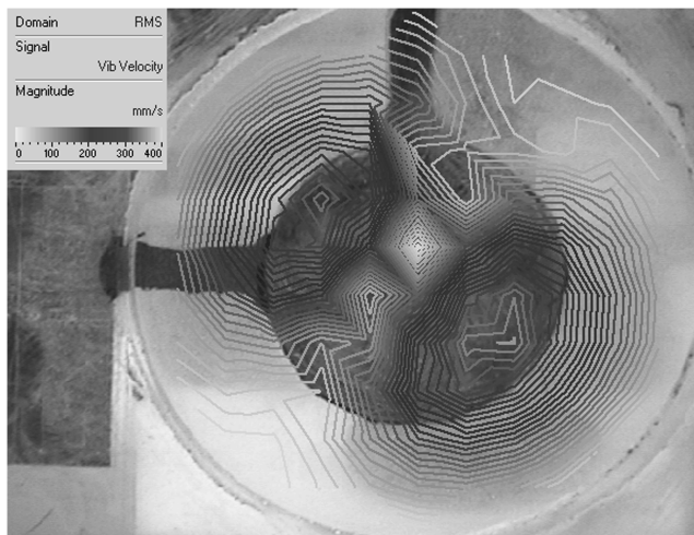
Fig. A16 Vibrometer scan at the fourth detected resonant frequency at 391 Hz excitation and 195.3 Hz vibration with a maximum rms vibrational velocity of 0.368 m/s at two points.
