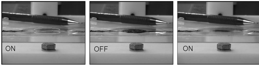
Fig. 4 Transverse vibration of membrane due to excitation at resonance (on-off-on sequence), with electrode border highlighted at the peak membrane displacements ( \pm ) in the leftmost image.
